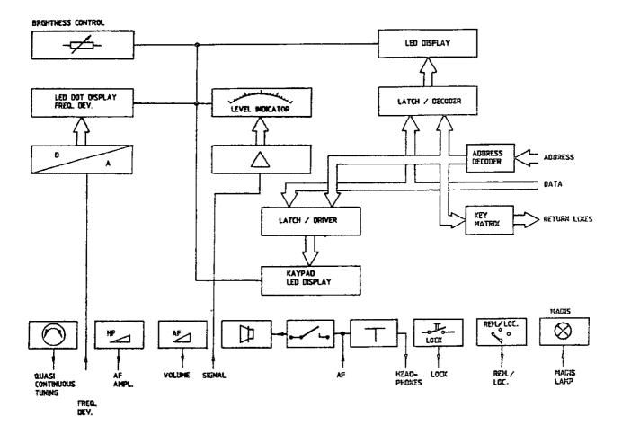
Fig. 5.1 Control Panel with LED Display (B3), Block Diagram
